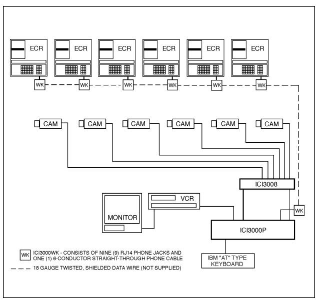
Figure 1. Typical ICI3000P System with Fixed Cameras
